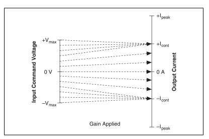
Figure 5. Input Voltage to Output Current Relationship for Periods of Time Greater Than 2.7 Seconds
